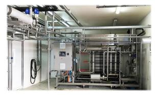
The fully automated GALAXIAS, has a power and automation panel with SIEMENS equipment (PLC series S7-1500) with a 12" touch screen. The pasteurizer is cleaned through its own cleaning circuit, optimizing uptime. The use of the equipment is continuously monitored through the central SCADA with corresponding maintenance alarms.
